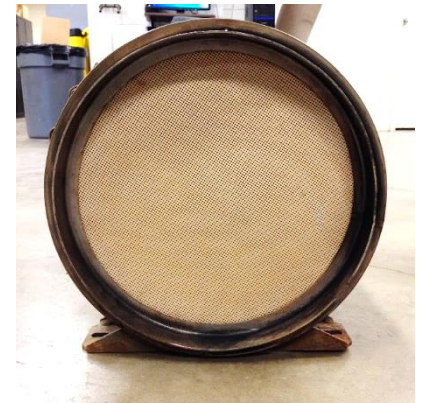
Outlet side of filter
